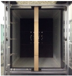
Figure 1. Test model in the wind tunnel
